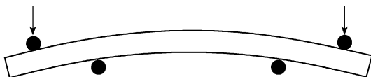
FIG. 3. Schematic representation of the four-point bending test. Arrows represent the direction of the force applied in bending to the tested stem. The deflection is measured via a graduated scale in a binocular microscope.
